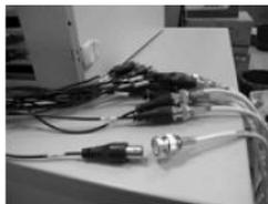
Fig. 2—3 Connecting video cameras to the BNC connectors
