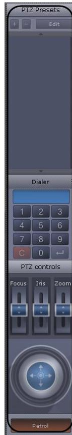
Fig. 5—4 The PTZ control panel
